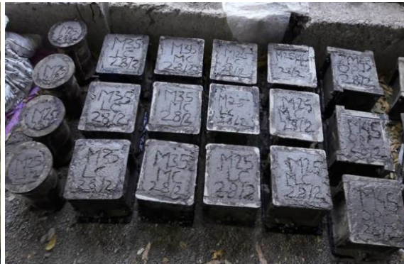
Fig. 2. Concrete cube and Cylinder of OPC, LC 3 and MC 3
