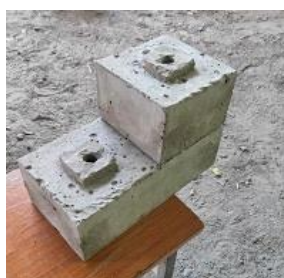
Figure 2. Hollow interlocking FaL-G bricks
