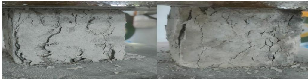
Fig.4 a) and b) Cubes showing after compressive strength test
