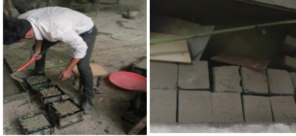
Fig. 1. Sample preparation and curing of test specimens
